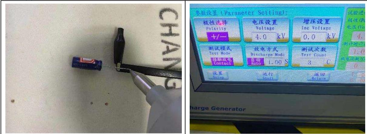
Fig 37. Direct Contact Discharge
